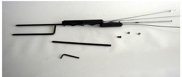
Insert threaded rod into support and slip on control modules Arrange as desired and secure with 1/4" nut. Bend stainless support for desired arrangement
